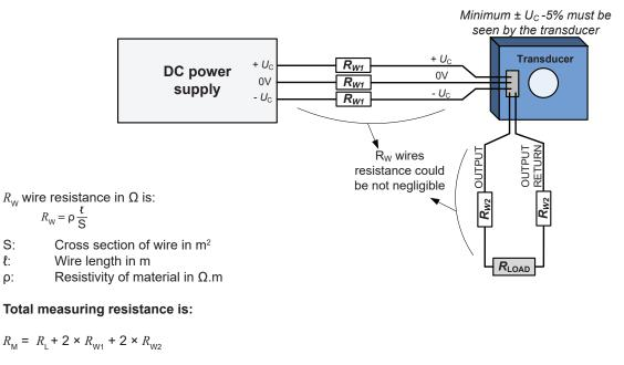
If  $R_{W1} = R_{W2} = R_{WIRE}$  then  $R_M = R_L + 4 \times R_{WIRE}$
